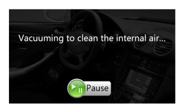
If there is refrigerant inside the hose, vacuum process will be stopped automatically.
