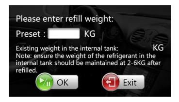
8) When refill running, LCD displays:
